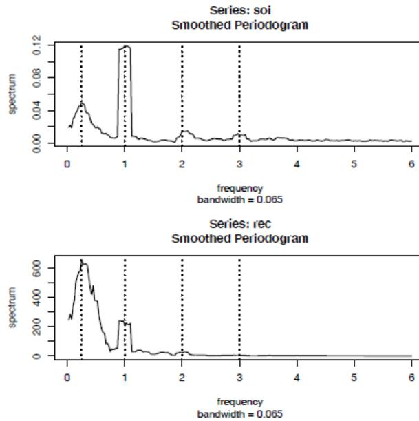
**Fig. 4.5.** The averaged periodogram of the SOI and Recruitment series  $n = 453$ ,  $n' = 480$ ,  $L = 9$ ,  $df = 17$ , showing common peaks at the four year period,  $\omega = \frac{1}{4}\Delta = 1/48$  cycles/month, the yearly period,  $\omega = 1\Delta = 1/12$  cycles/month and some of its harmonics  $\omega = k\Delta$  for  $k = 2, 3$ .
